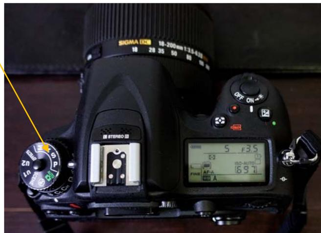
Top view of camera. From left to right; exposure control knob and LCD Screen shows typical settings.
