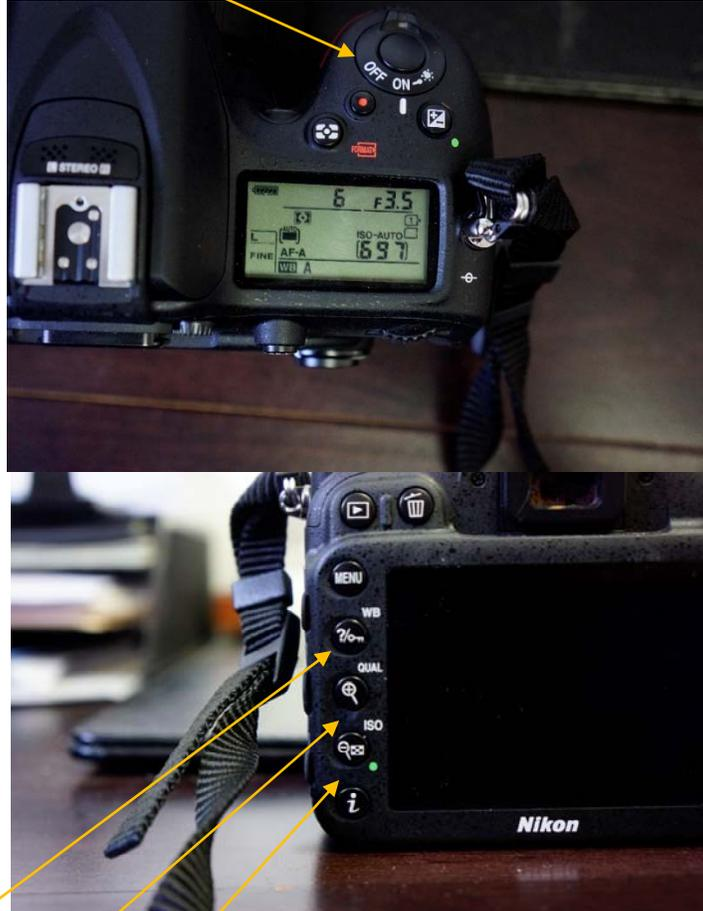
WB (White Balance), QUAL(ity) and ISO can be changed by pressing and holding buttons just to the lower left of writing on the camera
