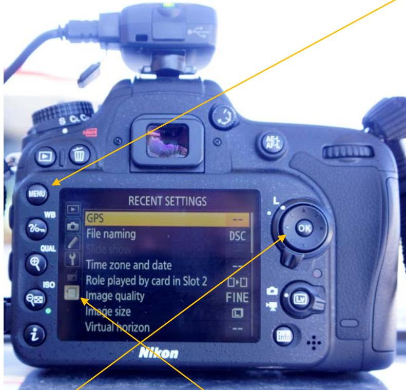
5. Using the “toggle” wheel highlight the “notepad” on the lower left of the screen.
