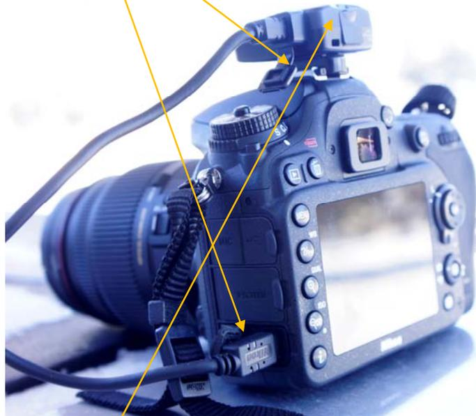
3. Turn the camera on. A **red light** will start blinking on the back of the GPS unit. Once a GPS signal lock has been achieved the light will turn to solid green (blinking green means that it almost has a good lock). You may need to take the camera outside with a clear view of the sky for about 5 minutes to get a good signal lock.
